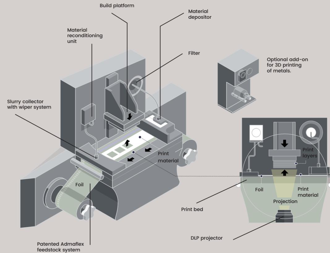
Featuring the unique capability of 3D printing both advanced ceramics and metals on one machine. This technology is ideal for functional and aesthetic parts requiring complex geometries, high resolution, fine details, and smooth surface while benefiting from excellent material properties.
