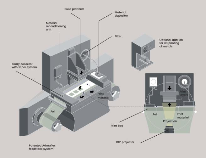
Featuring the unique capability of 3D printing both advanced ceramics and metals on one machine. This technology is ideal for functional and aesthetical parts requiring complex geometries, high resolution, fine details, and smooth surface while benefiting from excellent material properties.
