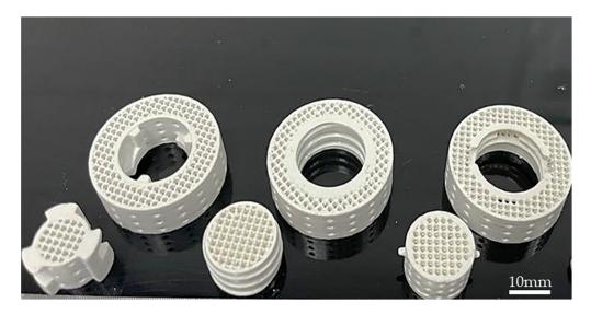
Figure 6. Green parts (from left to right: U-lock, Thread, Twist-lock).
