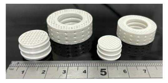
Figure 7. Green parts (left) and sintered parts (right).
