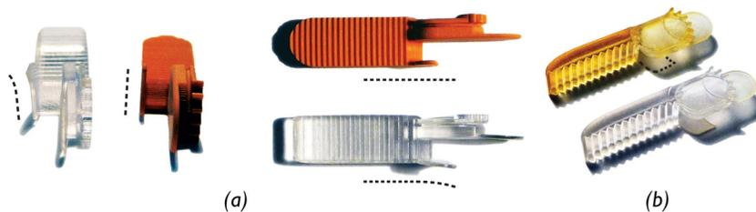
**Fig. 9** (a) Comparison of DragonFlex II and III grasper printouts showing the effect of material choice and printing orientation on the warpage of grasper flaps (curved dashed lines). (b) Old and new Accura<sup>®</sup> 60 grasper halves showing the impact of material's photosensitivity on its appearance (the new darker grasper on top gained a yellow hue) and increased brittleness (missing broken flap marked by a dashed contour).
