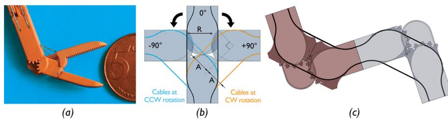
Fig. 2 (a) Real-scale 5 mm wide DragonFlex prototype tip. (b) Combined with the cable guiding profiles of radius  $R$ , the rolling joint equalizes the cable moment arms  $A$ . (c) Section through the basic modular parallelogram construction of DragonFlex joints (bent 90 deg). Adapted from Ref. [9].
