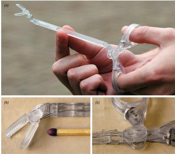
**Fig. 8** (a) Real-scale DragonFlex III prototype made from 3D Systems Accura<sup>®</sup> 60 and featuring (b) an innovative solution for cable-slack reduction and (c) a bolt-and-wheel mechanism for easy cable tensioning and fixation. (Reproduced with permission from Jelínek et al. [11]. Copyright 2015 by Informa Healthcare).
