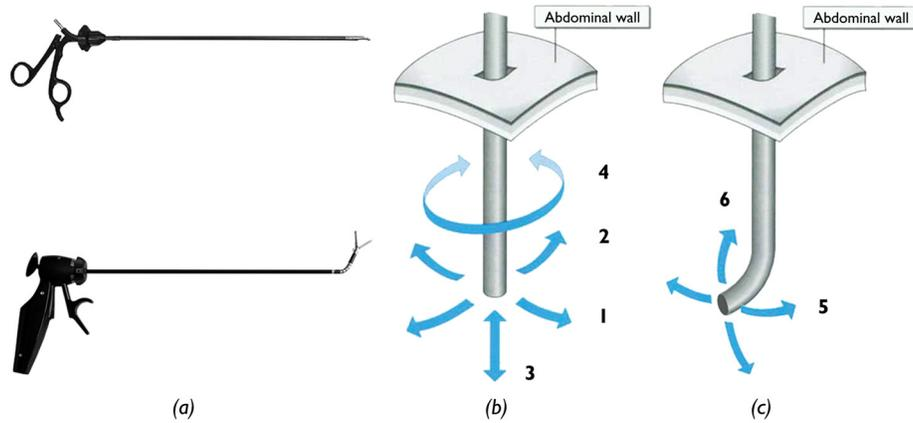
Fig. 1 (a) Rigid [6] and steerable [7] laparoscopic instruments; (b) rigid instrument DOF [8]; and (c) additional steerable tip DOF [9]
