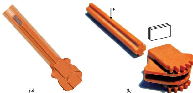
**Fig. 6** (a) Inner rod and slot in DragonFlex II accommodating a compression spring for cable tensioning. (Reproduced with permission from Jelínek et al. [11]. Copyright 2015 by Informa Healthcare). (b) Breakage of the inner rod due to force  $F$  applied along the printed layers, demonstrating the importance of choosing an optimal printing orientation.
