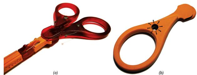
**Fig. 7** (a) Replacement of several NanoCure RCP30 DragonFlex II components by the more flexible and creep-resistant NanoCure R5 alternative. (b) The location of the loosened cable-fixing bolt, originally having an interference fit with the handle, due to permanent radial expansion of the hole.
