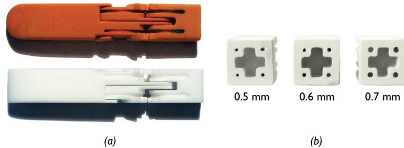
**Fig. 10 (a) Comparison of DragonFlex II and IV grasper printouts demonstrating the shrinkage of solid long and thin features (grasper flaps) made from the alumina–zirconia composite. (b) The effect of sintering on hollow long and thin features (cable holes) shrinking to 0.36, 0.39, and 0.58 mm in diameter from the designed 0.5, 0.6, and 0.7 mm, respectively.**
