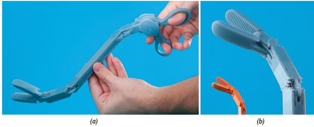
**Fig. 3 (a) Upscaled Objet VeroBlue™ DragonFlex I prototype demonstrating tip opening and pivoting in 2DOF. (b) Close-up picture highlighting the striking size difference between the 5 mm and 15 mm wide prototype tips. Adapted from Ref. [9].**
