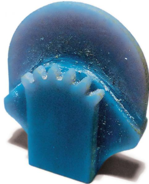
**Fig. 4 Upscaled DragonFlex I joint component made from Objet VeroBlue™ showing the wear of the outermost sticky coating and some sign of oxidation**
