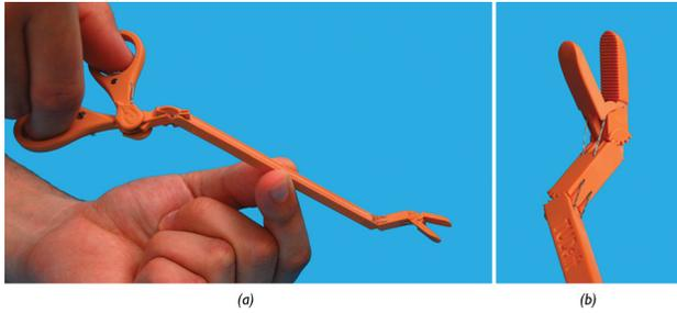
**Fig. 5** (a) Real-scale DragonFlex II prototype made from EnvisionTEC<sup>®</sup> NanoCure RCP30. (b) Close-up on the tip showing cable-driven joints and grasper. Adapted from Ref. [9].
