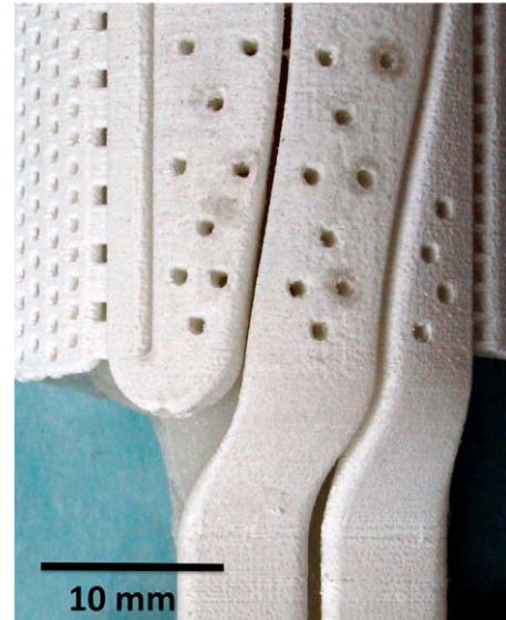
Fig. 3. Silica ceramic component built by stereolithography.
