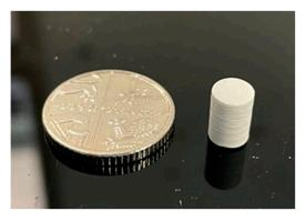
Figure 1. Digital Light Processed green sample.
