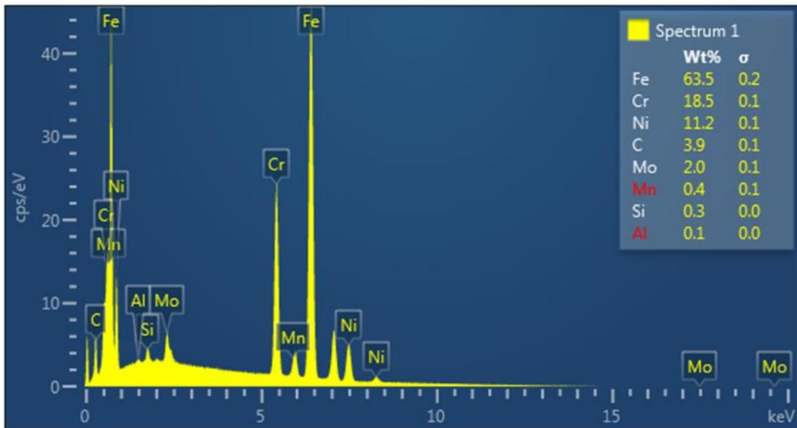
Figure 7: Composition of a sintered 316L DLP printed body.
