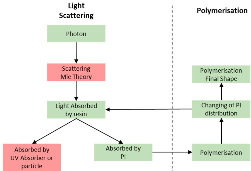
**Figure 2:** Different aspects of light penetration in slurries for the DLP process.
