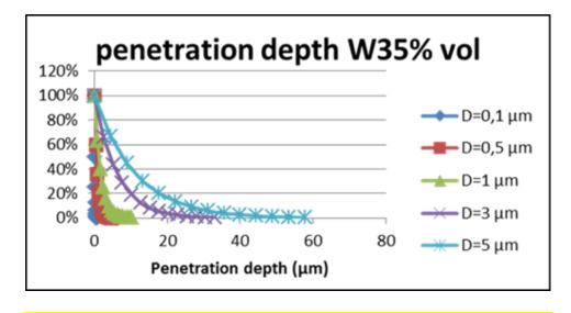
Figure 4: Penetration depth of light depending on particle size of absorbing powder.
