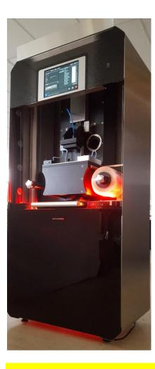
Figure 9: Admetalflex 130 (for printing metals).
