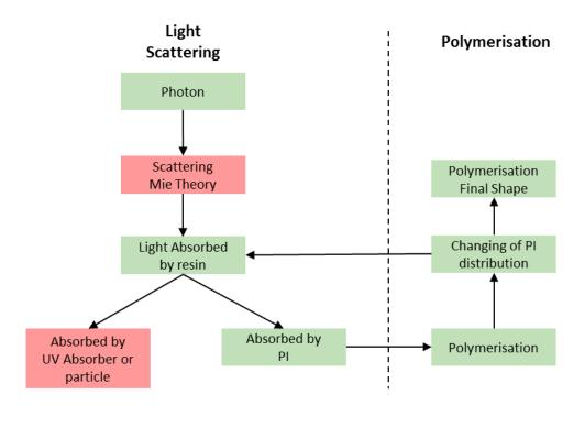
Figure 2: Different aspects of light penetration in slurries for the DLP process.
