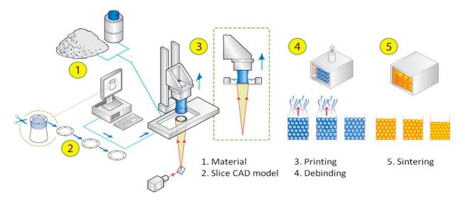
Figure 1: Process of DLP printing of ceramics or metals.
